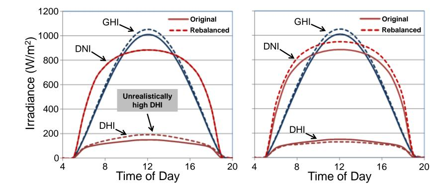
Improper rebalancing can skew PV energy simulations (PVsyst & SAM)
