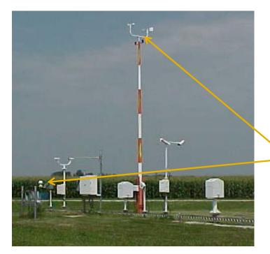
Standard surface observations are taken at 2 meters for dry bulb temperature and 10 meters for wind speed and direction.
