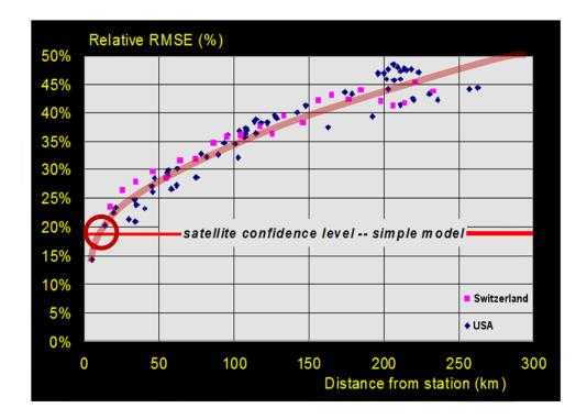
Ground data are suitable at distances up to 10-25 km from project site (can be <5 km in regions with variable topography)
